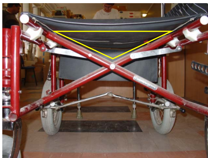
Figure 56. The space for the fundament device under the seat of the B4205 transit lying wheelchair
