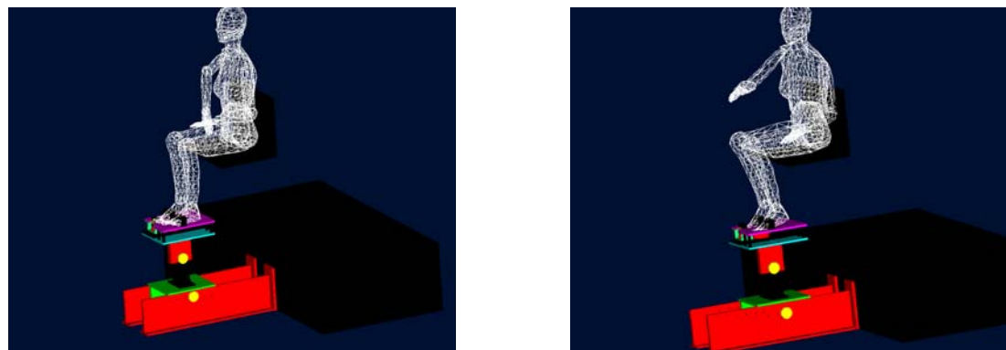
Figure 61 Concept ADD_FBT_v1 for position 1 (left) and position 2 (right) with 25 percentile female mannequin.
