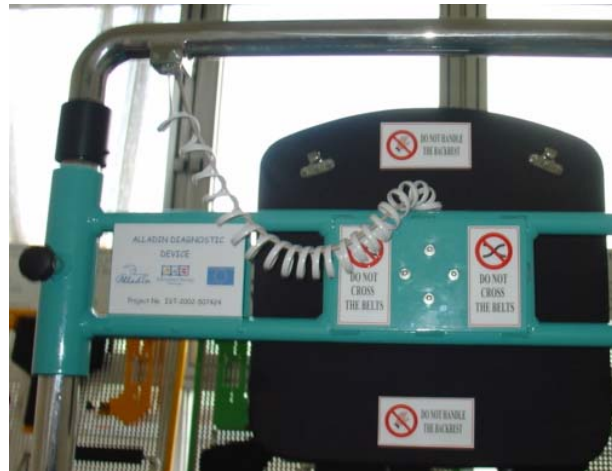
Figure 45. Leading the cable from the trunk sensor to the trunk frame
