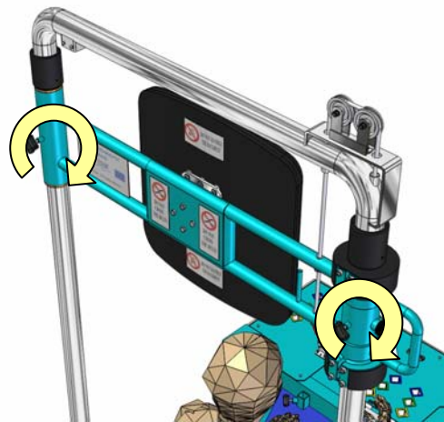
Figure 39. Two screw clamps fix the backrest framework
