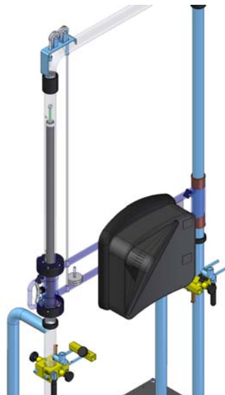
Figure 40. Counterbalancing rod slides inside the trunk frame
