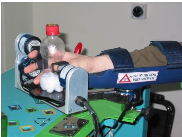
Figure 5: The ALLADIN Finger Device integrated with the ALLADIN Arm Device
