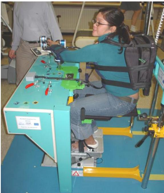
Figure 9: Isometric force-torque measurement in progress in the Maria Middelaers Hospital
