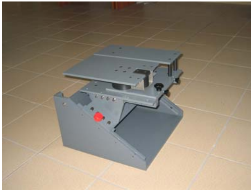
Figure 6. Mock-up in PVC of the first version of the foot platform
