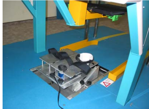
Figure 10. The foot platform integrated into the ADD (Alladin Diagnostic Device) with sensors, hell support and steps.
